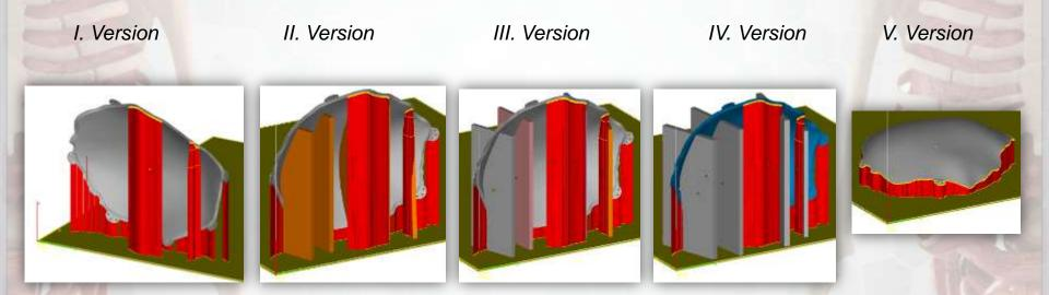
For each version the position of the part (cranial implant) was changed with specific change of support material and removed after heat treatment. Support/ Part Exposure Parameters" were not changed, these parameters were identical for all versions.
